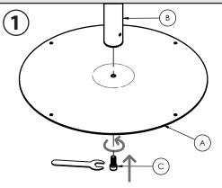
Step 1: Screw the M10 bolt into the upright, clamping the base in place.
